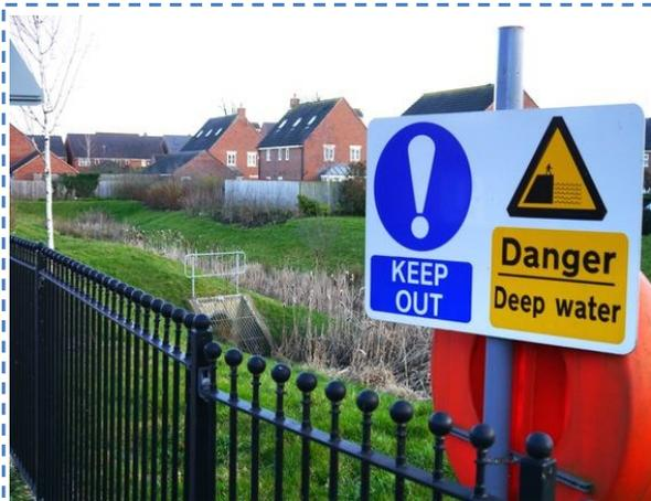
POORLY DESIGNED SUDS CAN RESULT IN RESTRICTED ACCESS TO RECREATION AREAS DUE TO SAFETY ISSUES. IF DESIGNED MORE APPROPRIATELY THEN FENCING WOULD NOT BE REQUIRED.
