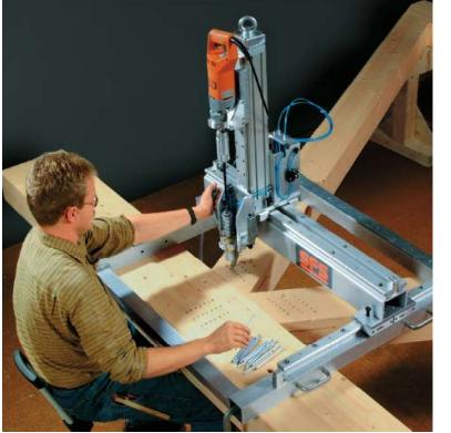
Fig. 7. Typical factory assembly using dowels
