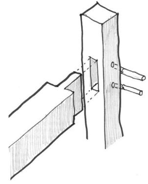
Fig.2. Mortice and tenon joint
