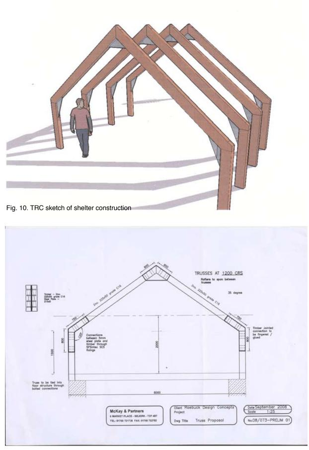
Fig. 11. Structural Engineer's section drawing for shelter construction
