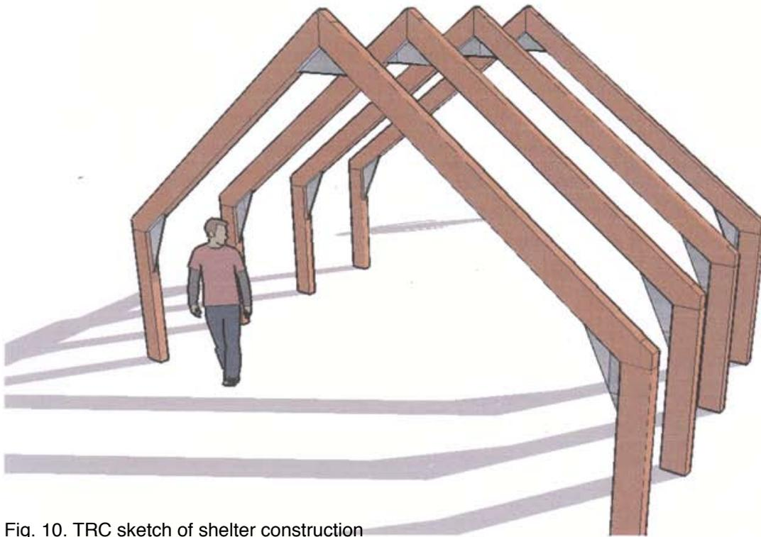
Fig. 10. TRC sketch of shelter construction
