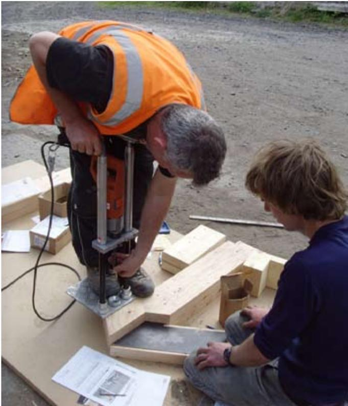
Fig. 12. Using proprietary drill to line up and insert first dowel on test rig
