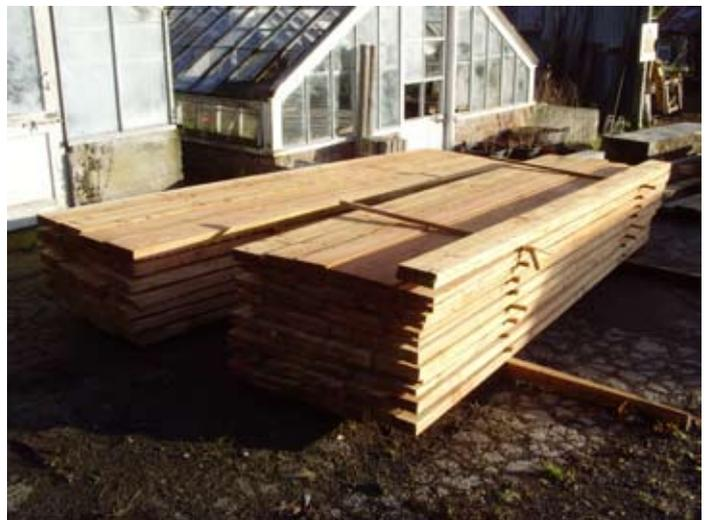
Fig. 17. Milled timber with structural posts and rafters (left) and cladding/sarking boards (right)
