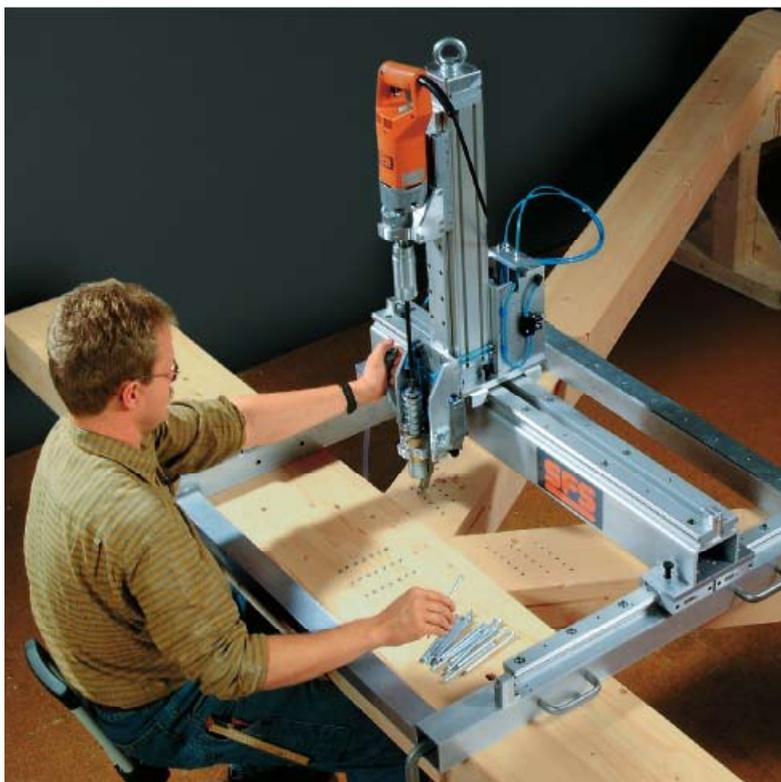
Fig. 7. Typical factory assembly using dowels
