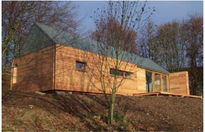
**Timber sources** : The timber frames are untreated Scottish softwood in prefabricated panels supplied by ARM Buildings. Douglas fir beams and European larch supplied by local sawmill, Abbey Timber. Scots Pine glulam post and beam supplied by Norbuild of Forres. Redwood windows and external doors from various sources.
