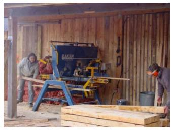
Figure 3. sawn boards passing through planer-thicknesser
