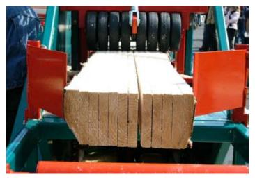
Figure 2. sawn log passing through multi-blade saw
