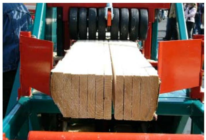
Figure 2. sawn log passing through multi-blade saw
