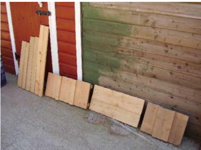
Figure 7. typical cladding profiles and examples of surface coatings
