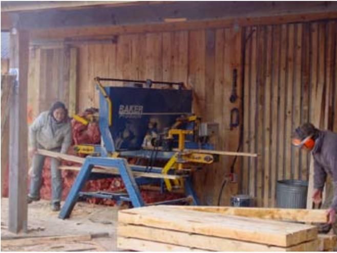
Figure 3. sawn boards passing through planer-thicknesser
