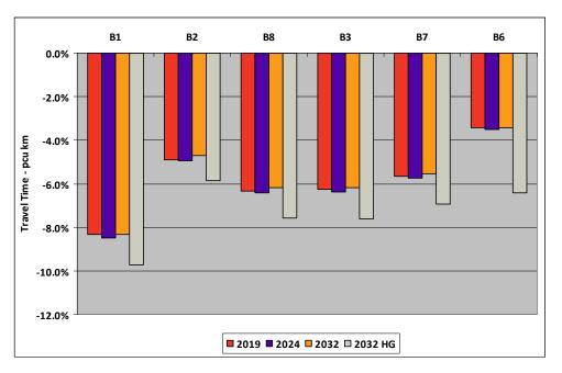
Figure 7.10 Modelled change in total travel time, % change versus Reference Case
