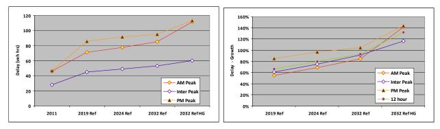
Figure 7.6 Modelled delay (vehicle hours) and % change from 2011
